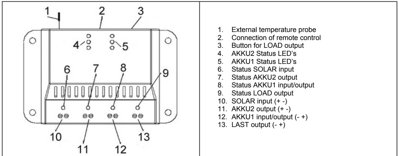
**Attention:** In case of reverse connection to the load output, devices without own protection may be destroyed. Every single consumer must be protected individually by its own fuse.
